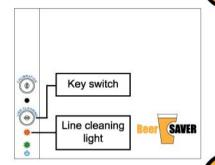
Turn the line cleaning key clockwise. The **orange** light will turn on.
